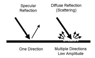
Due to surface roughness, reflected radio waves can be scattered in many directions.
