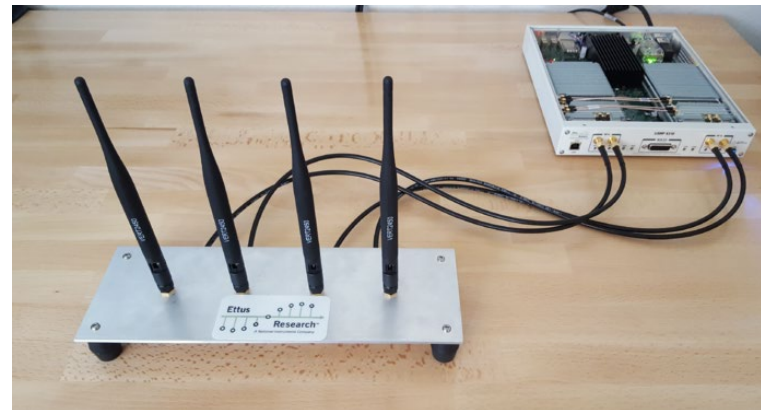
USRP with four vertical antennas
