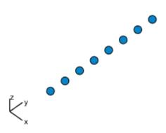
Aperture Size: Y axis = 42.827 mm Element Spacing: Δ y = 5.353 mm Array Axis: Y axis
