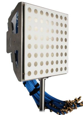
Aurora C-Band Massive MIMO array 64 elements, 5-6 GHz https://www.taoglas.com/
